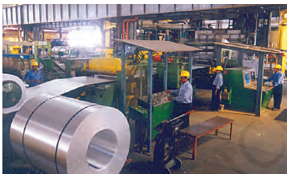
Fig. 6.3: Strip coating mill at smelter of NALCO
