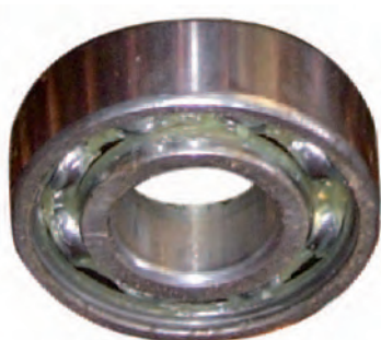
Fig. 9.16 : Ball bearings reduce friction
