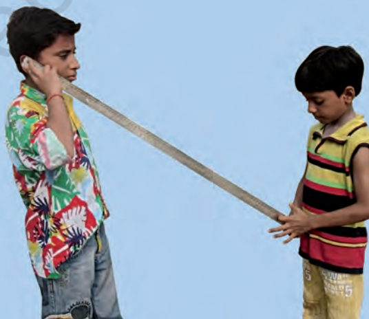
Fig. 10.12 : Sound travelling through a metre scale
