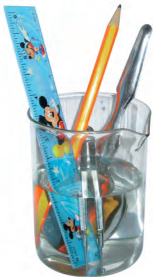
Fig. 3.8 Conduction of heat by different materials
